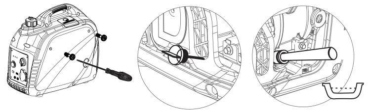
Do not tilt generator when adding oil. This could result in overfilling which could damage CAUTION! the engine. CAUTION! Make sure no foreign matter enters the crankcase
